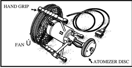
The TURBAIR ELECTRAFAN is an air-assisted spinning disc sprayer for low and ultra-low volume application of insecticides and fungicides in situations with no natural air movement, e.g. indoors. The ELECTRAFAN produces small even sized droplets which are carried in the airstream to the target.
