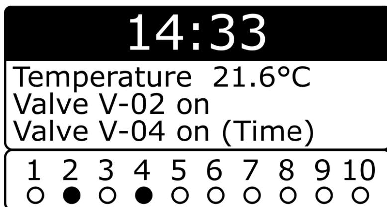
In the top line the actual time is displayed. As soon as an alarm is detected a flashing alarm sign is displayed in the top right corner of the screen.
