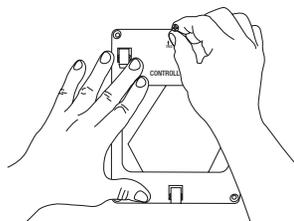
4. Install a wall anchor in the marked position then install the bracket onto the anchor using one of the mounting screws provided (do not tighten screw fully yet). The center screw will automatically level the bracket on the wall. After level is set, mark the other mounting holes and install the remaining wall anchors.
