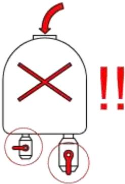
Before filling the tank, close the tank drain valve and open the pump feed line valve! The tank takes up to 400 Liters (100 gal).
