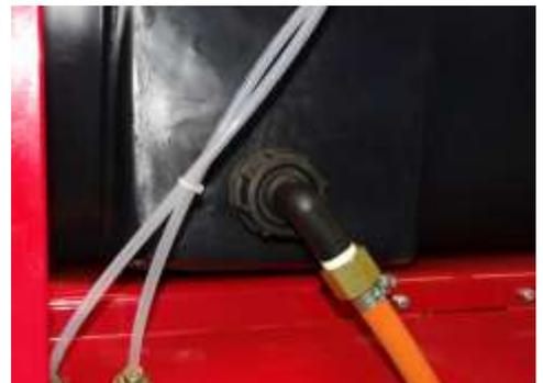
Hydraulic agitator mounted on tank
