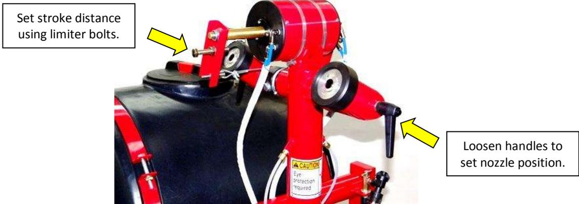
The reversion system requires compressed air from the unit's blower to operate. Run the unit to try and set the reversion stroke distance and nozzle position.
