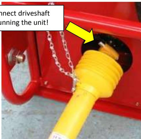
Correct mounting of the driveshaft. Fix chains to prevent guard from rotating.
