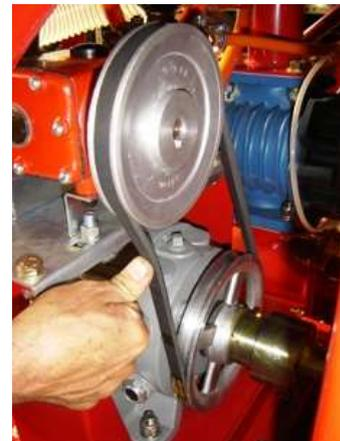
Checking the pump belt.
