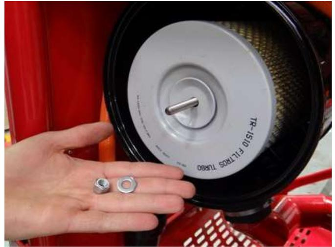
To remove element release nut.
