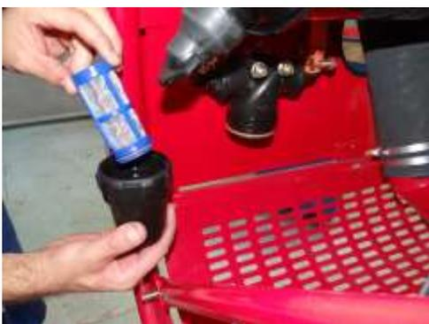
For cleaning the formulation filter, shut the valve, unscrew the filter cup and clean the strainer. Remember to open the valve after reassembling the filter.
